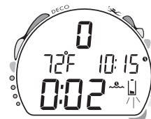
Fig. 9 -Low Battery Condition
