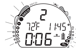
Fig. 50 - Viola Gauge Mode (on Surface)
